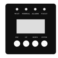
Check all connections again before starting the inverter. To start the inverter, please switch on AC breaker first, then switch on the DC switch (If there) on inverter. If all connections are correct and PV configurations are correct, LCD will be on, "WAIT" LED will be on, inverter will be standby for Grid-tied connecting.
