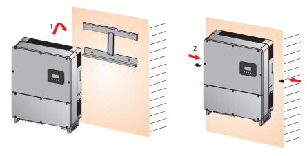
2.4 Hang the inverter on the screws, check right and left sides, make sure the it is hung in the right position, then screw the screws tight.
