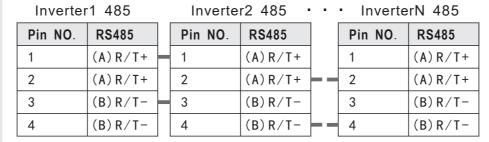
**Note:** When the network communication is for more than two (including) inverters, for last inverter, the 2P dial switch next to RS485 terminal can be switched to "ON", equivalent to add a  $120\Omega$  communication terminal resistance between the R/T+ and R/T-.
