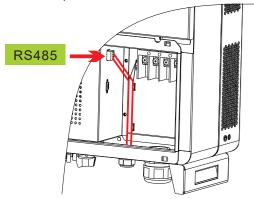
**Note:** After connecting the 485 communication line, fix the cable on the tie bridge to avoid loosening and falling off the communication line.
