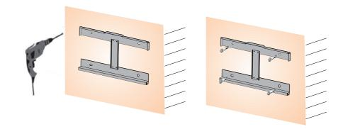
2.3 Hang the inverter gently up and hung on the rack, check and ensure that both sides are fixed in the correct position, then tighten the screws at both ends (attached in accessoriesbag).
